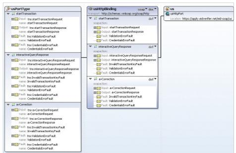
for an XMLBeans implementation, which was then compiled as a Java service class. Once the elDverifier service was exposed, XFire automatically generated a WSDL – the WSDL is shown below in the XMLSpy graphical WSDL editor.
