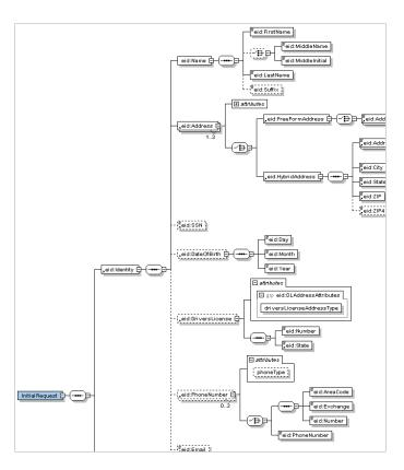
This data type definition provides the syntax, and dictates the structure, for the data that is transmitted by the elDverifier Web service.
