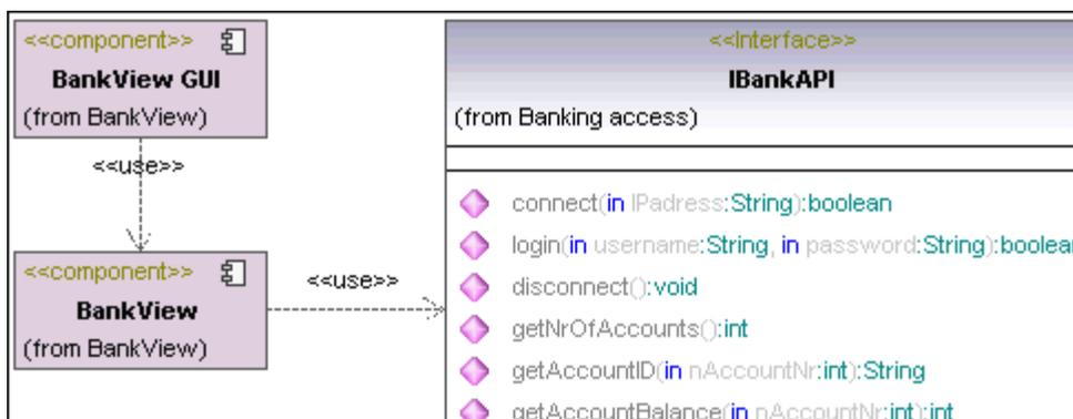
The usage dependency (<<use>>) connects a **client** element to a **supplier** element. In this case the IBankInterfaceAPI interface uses the services of components BankView and BankView GUI.
