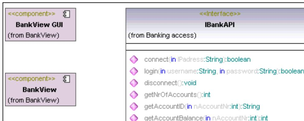
The BankView component is the component produced by the "forward-engineering" process described in this tutorial.
