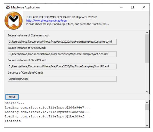
If Eclipse encounters system configuration or run-time errors, you will be prompted, see also <u>Handling JDBC</u> references 1042. Otherwise, the Java application executes the mapping transformation and generates the **CompletePO.xml** at the output path (in this example, the output path is **C:\codegen\Java\CompletePO**).
