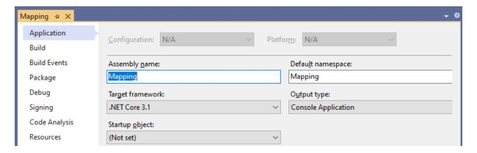
The default name of the generated application is **Mapping**. Optionally, you can change this and other settings before generating code, from the <u>Mapping Settings</u> dialog box.
