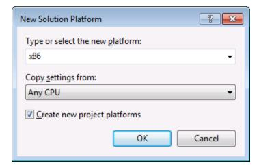
You are now ready to build and run the solution in Visual Studio. Remember to build using the configuration that matches your target platform (x86, x64); otherwise, runtime errors might occur.
