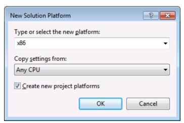
You are now ready to build and run the solution in Visual Studio. Remember to build using the configuration that matches your target platform (x86, x64).
