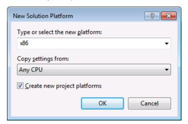
You are now ready to build and run the solution in Visual Studio. Remember to build using the configuration that matches your target platform (x86, x64); otherwise, runtime errors might occur.
