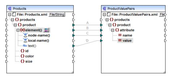
Fig. 7 Mapping XML element names to attribute values (in MapForce)
