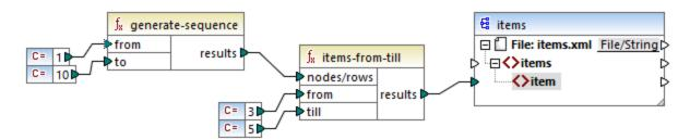
Because the **from** and **till** arguments are set to **3** and **5**, respectively, only the subset of values from **3** through **5** are passed on to the target. Consequently, the mapping output is as follows (excluding the XML and schema declarations):
