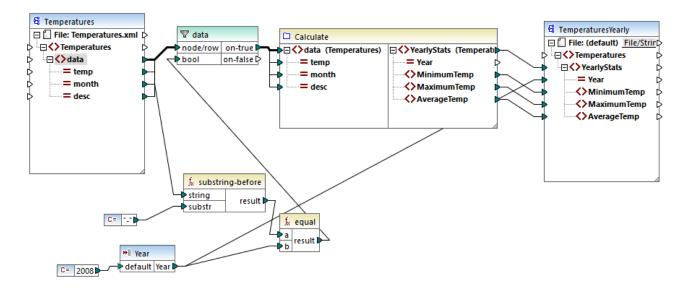
The mapping above illustrates a typical case of a UDF that operates on a set of values and thus requires all the input values in one call. Specifically, the **Calculate** user-defined function returns the minimum, maximum and average temperatures, taking as input data from a source XML file. The expected mapping output is as follows:
