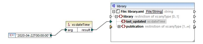
In the mapping illustrated above, a string constant ("2020-04-28T00:00") has been used to provide the input argument of the function. The input could also have been obtained from an item in the source document. The xs:dateTime function returns the value 2020-04-28T00:00:00 of type xs:dateTime.
