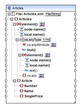
In the component above, notice there are two element() nodes. The second element() node provides dynamic access to grandchildren of the <articles> node in the **Articles.xml** instance.
