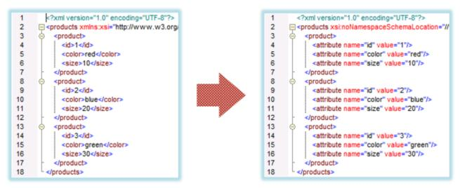
Fig. 6 Mapping XML element names to attribute values (requirement)
