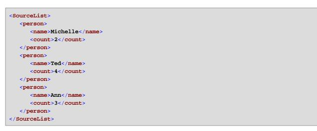
With the help of the **replicate-item** function, you can repeat each person name a different number of times in a target component. To achieve this, connect the **count** node of each person to the **count** input of the **replicate-item** function:
