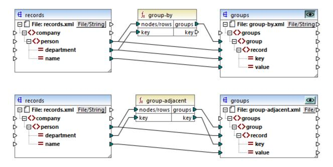
According to the rules, the default processing order of this mapping in MapForce Server and in generated code is from top to bottom. You can check that this is the case by generating XSLT 2.0 code, for example.
