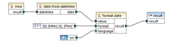
Note that the mapping above is designed for the Built-in, C++, C#, or Java transformation languages. In XSLT 2.0, the same result can be achieved by the following mapping:
