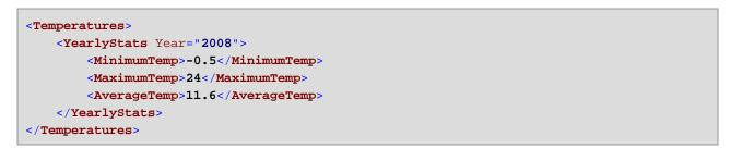
As usual, the mapping execution begins with the top item of the target component (**YearlyStats**, in this example). To populate this node, the mapping attempts to obtain source data from the UDF, which in its turn, triggers the filter. The filter's role in this mapping is to pass onto the UDF only temperatures from year 2008.
