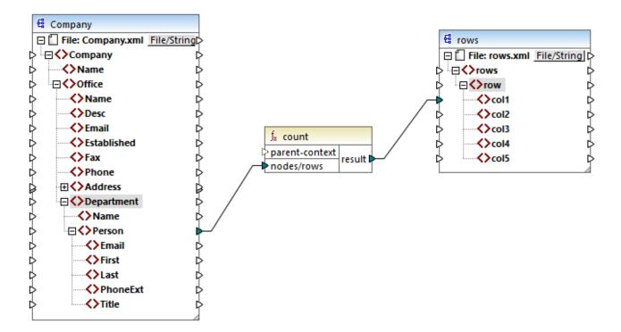
In the source XML of the mapping above, there is a single **Company** node which contains two **Office** nodes. Each **Office** node contains multiple **Department** nodes, and each **Department** contains multiple **Person** nodes. If you open the XML file in an XML editor, you can see that the distribution of people by office and department is as follows:
