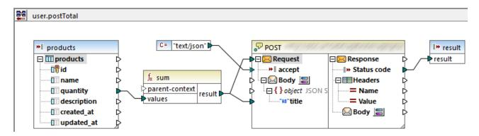
Normally, aggregate functions like sum, count, etc produce a single value. Nevertheless, if there is a parent connection that allows it, they may produce a sequence of values as well, as described further in the Example: Changing the Parent Context<sup>404</sup>.
