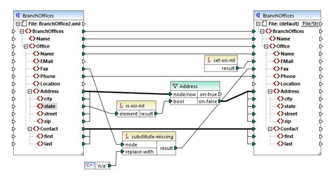
As illustrated above, the **is-xsi-nil** function checks whether the xsi:nil attribute is "true" for the **state** item in the source file. If this attribute is "false", the filter will copy the parent **Address** element to the target. The source XML file looks as follows (excluding the XML and namespace declarations):
