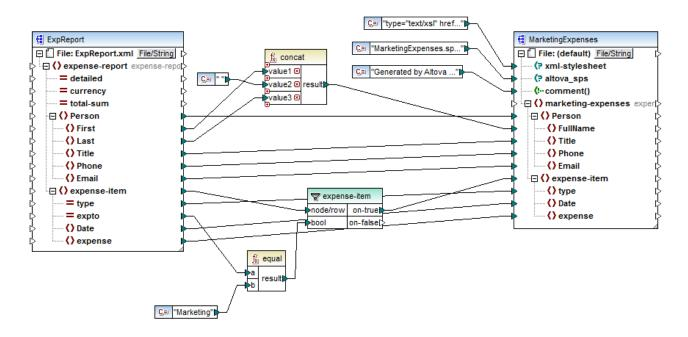
As shown above, the mapping reads data from a source XML which contains an expense report ("ExpReport") and writes data to a target XML ("MarketingExpenses"). There are several other components between the target and source. The most relevant component is the **expense-item** filter ( $\overline{T}$ ), which represents the subject of this topic.
