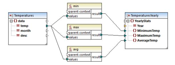
As a rule of thumb, the input data (sequence or non-sequence) determines how often the function is called:
