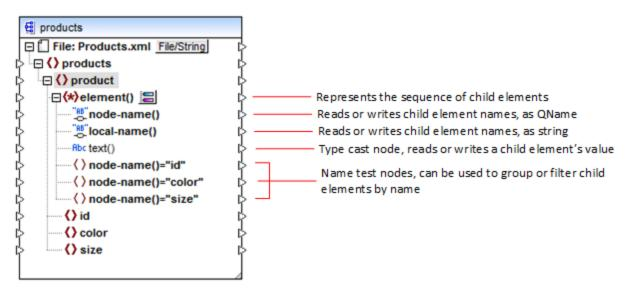
Fig.3 Enabled dynamic node names (for elements)
