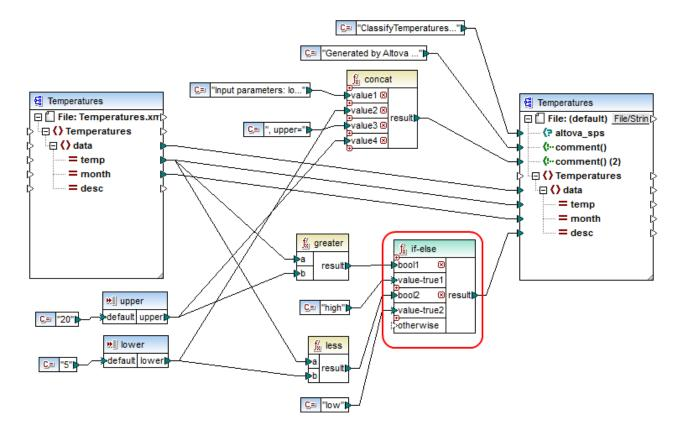
This mapping reads data from a source XML which contains temperature data ("Temperatures") and writes data to a target XML which conforms to the same schema. There are several other components between the target and source, one of them being the **if-else** condition (highlighted in red), which is also the subject of this topic.
