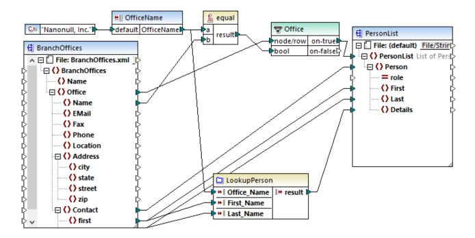
In the mapping above, both the source and the target component are XML. The source XML file contains two **Office** elements.
