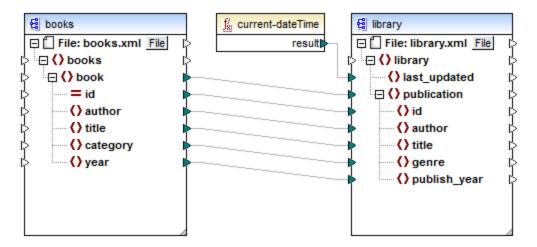
2. When you draw a connection *to* a target item, the mapping generates instance data of that kind. If the source item contains simple content (for example, string or integer) and if the target item accepts simple content, MapForce copies the content to the target item and, if necessary, converts the data type. Zero, one, or multiple values can be generated, depending on the incoming source data, see the next bullet.
