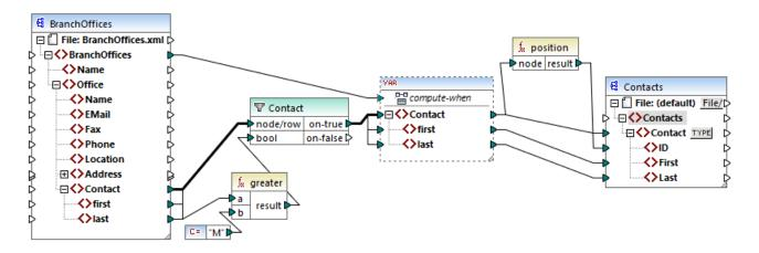
The result of variables in MapForce are always sequences. Therefore, in the mapping above, the **position** function iterates through the sequence created by the variable and returns the position of each item in that sequence. This mapping is discussed in more detail in <u>Example: Filtering and Numbering Nodes</u><sup>(15)</sup>.
