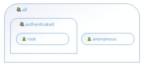
As the diagram shows, every user in the system inherits the privileges defined in the all role. However, only existing users (in this case, aroot) inherit the privileges defined in the authenticated role. If you add any new users to FlowForce Server, they are automatically assigned to the all and authenticated role (and thus granted the privileges defined in those roles, if any), as follows.
