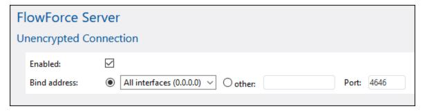
2. Make sure that FlowForce Server is allowed to communicate through the operating system's firewall. In this example, since the "Apollo" FlowForce Server runs on Windows, it must be allowed to communicate through Windows Defender Firewall.
